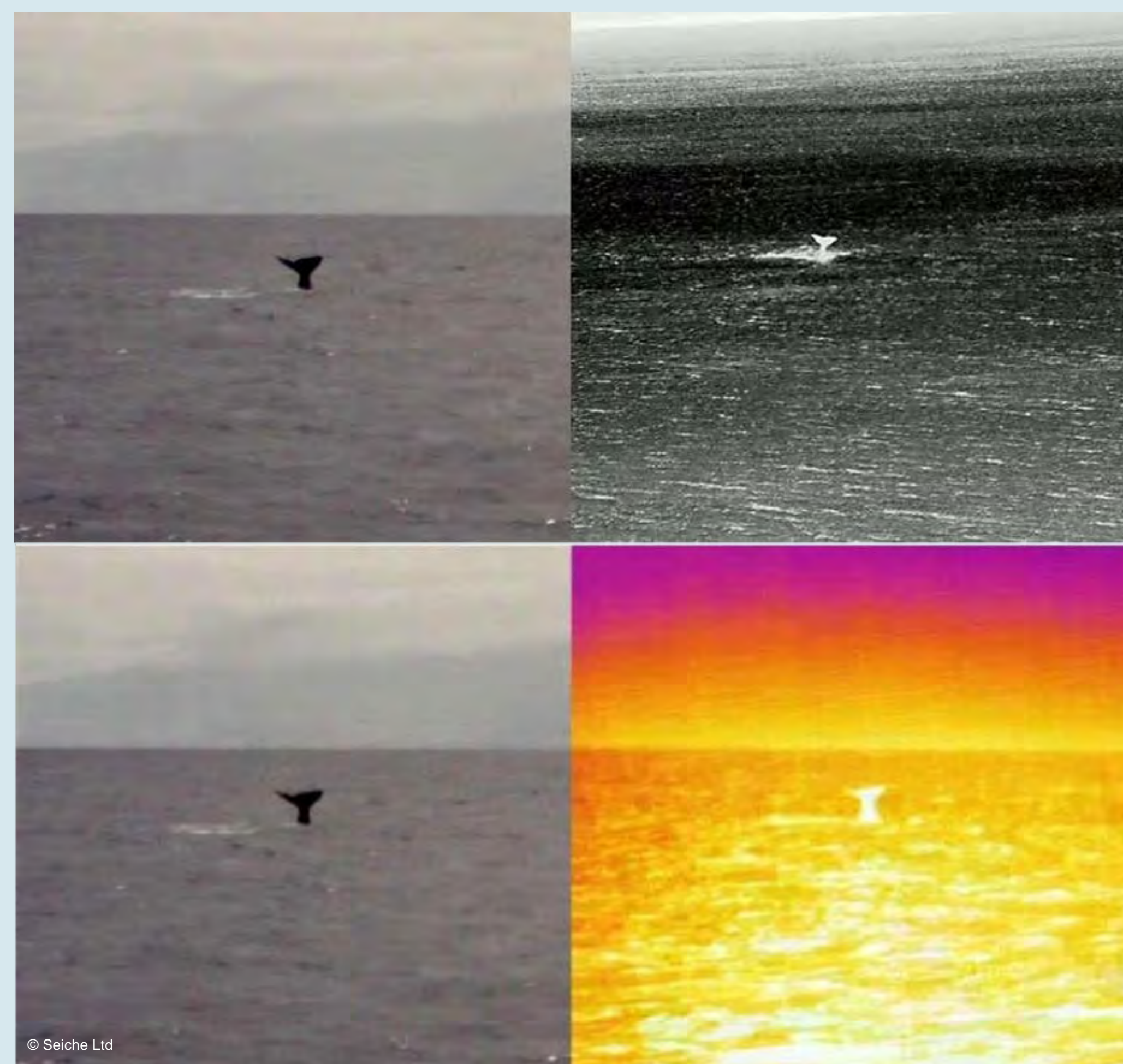
Example of dual camera system - sperm whale fluke on HD / thermal imaging camera
