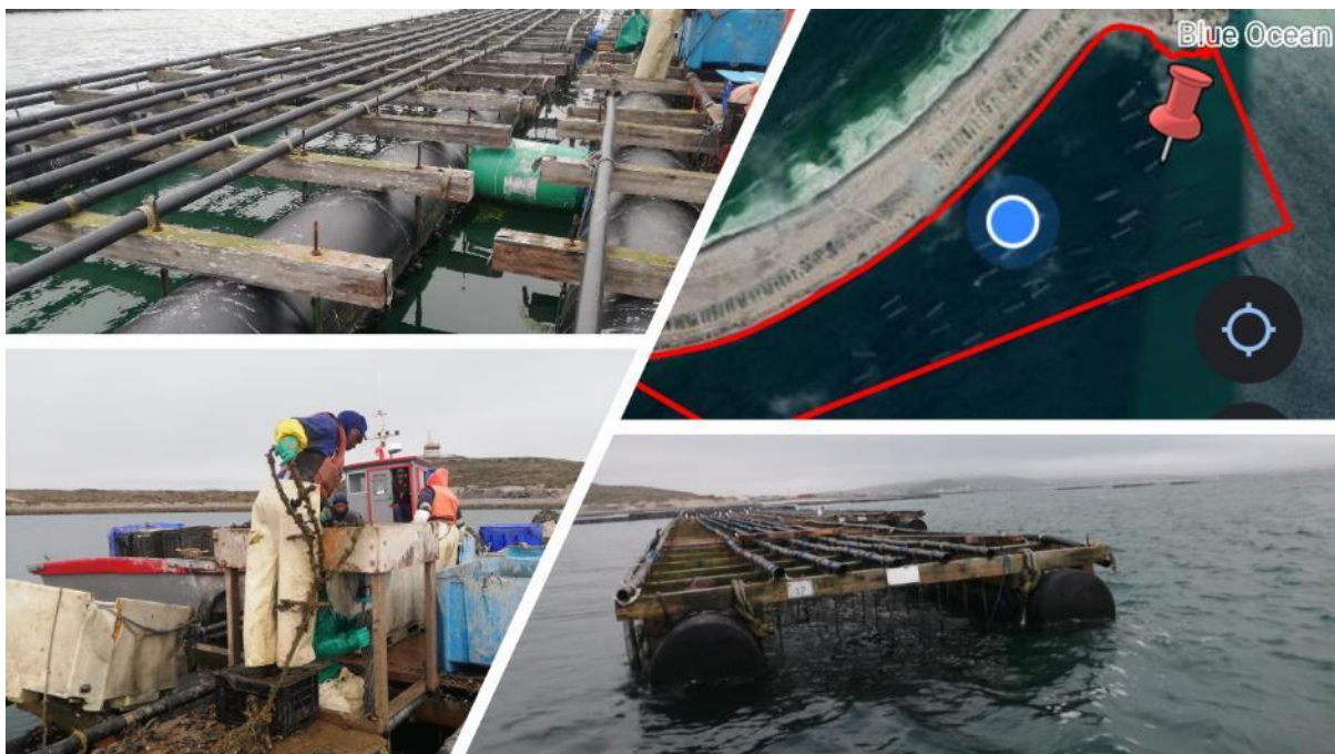
Figure 5. (Top left) BOM rafts in good condition but lashed together while awaiting their own moorings; green drums placed between rafts to reduce damage by rafts buffeting against one another. (Top right) Live Google Earth pin of location of compliance photograph in relation to BOM, Small Bay licence area (red boundaries). (Bottom left) Operators seeding droppers with mussels. (Bottom right) Raft 17 in good condition, facing the prevailing current and swell, suitably marked, and on its own moorings.
