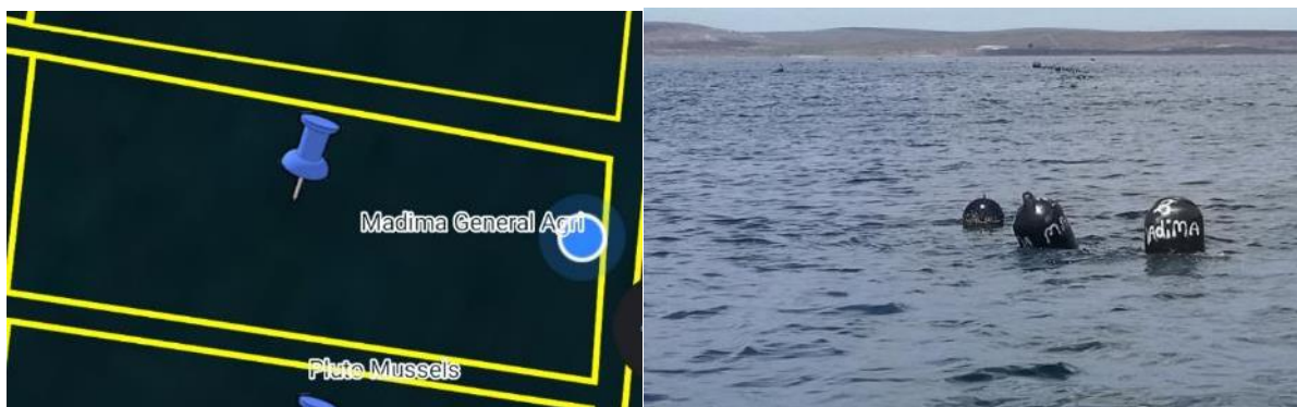
Figure 10. (Left) Live Google Earth pin of location of compliance photograph in relation to Madima licence area (yellow boundaries). (Right) Infrastructure are marked with unique identifiers, lines are taught and not overloaded.
