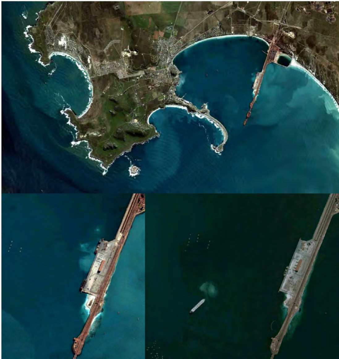
Figure 6.22. Turbidity generated under high wind conditions (top) and by propeller wash (bottom) in Saldanha Bay (Source: van Ballegooyen et al. 2012).
