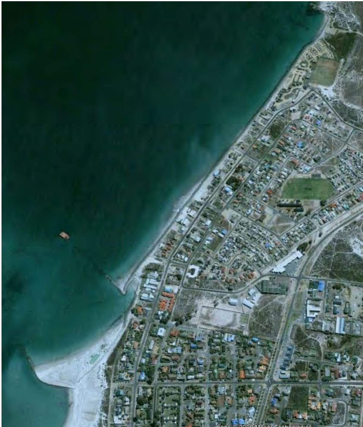
Figure 7.7. Langebaan Beach as it is at present (2020), with groynes extending out perpendicularly from the shore on the lower (southern) end of the image and rock revetment extending all along the shore from the uppermost groyne towards the upper end of the image.
