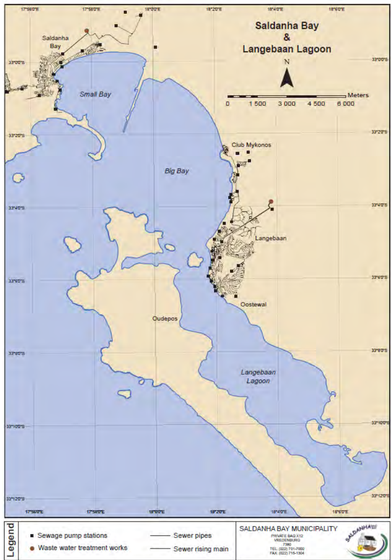
Figure 3.18. Location of wastewater treatment works, sewage pump stations and sewer pipes in the Saldanha and Langebaan area in 2014 (Source: Saldanha Bay Municipality, Elmi Pretorius 2014).
