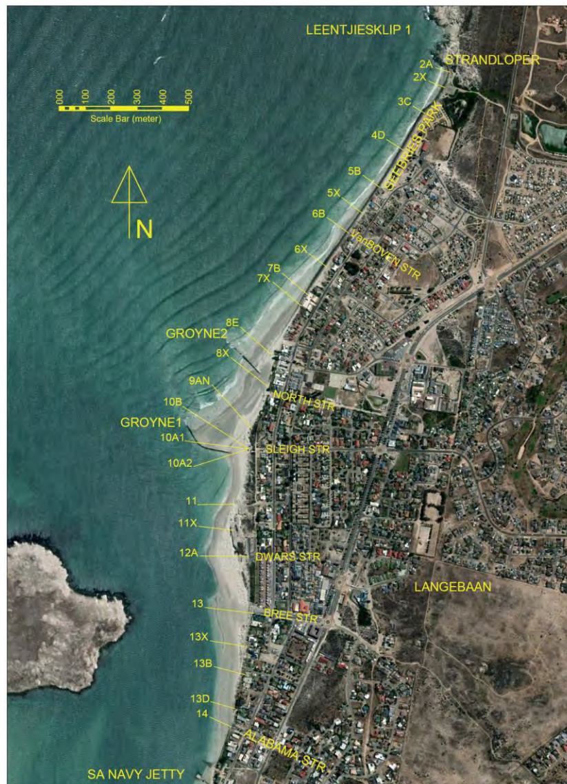
Figure 7.8. Erosion monitoring sampling sites in Langebaan between Leentjiesklip 1 (Strandloper restaurant) and Alabama street (SBWQFT 2019).
