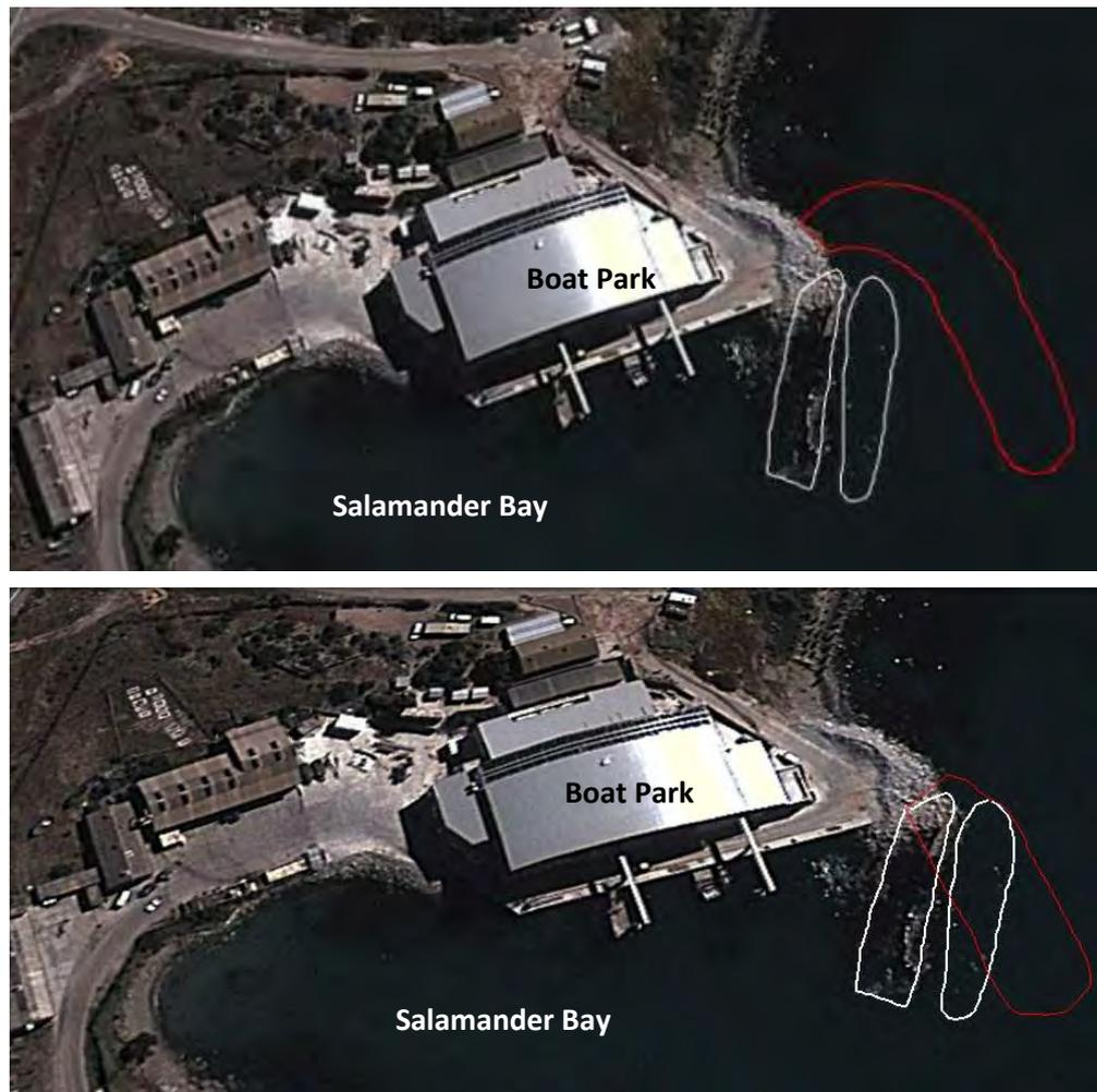
Figure 3.13. Bird's eye view image of Salamander Bay showing the existing boat park, the two shipwrecks (white) and the site of the proposed breakwater (red). The breakwater may either be positioned A) on the outside of the two shipwrecks, or B) on top of sections of the shipwrecks.
