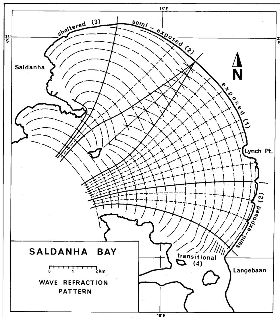
Figure 6.2 Predicted wave field in Saldanha Bay showing wave height and direction prior to harbour development (Source: Flemming 1977).
