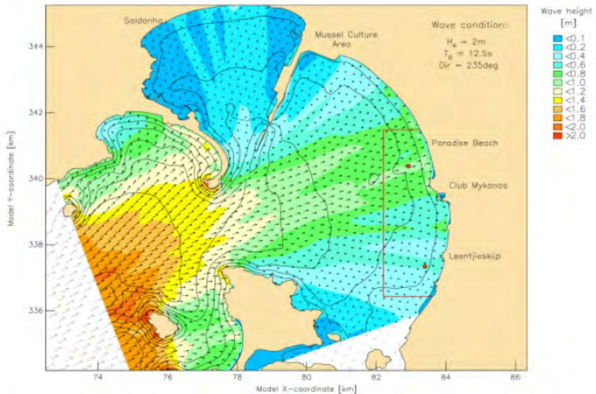
Figure 6.3 Predicted wave field in Saldanha Bay showing wave height and direction after the construction of the causeway and the iron-ore Terminal (Source: WSP Africa Coastal Engineers, 2010).
