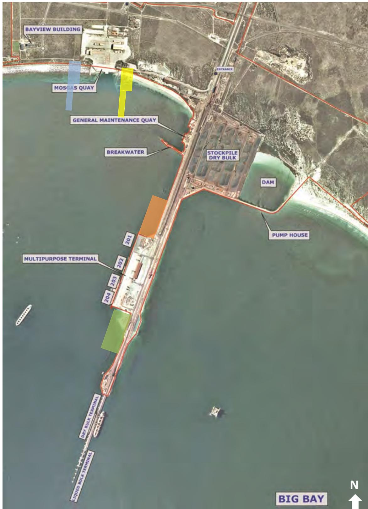
Figure 3.13 The iron ore terminal (IOT), the multi-purpose terminal (MPT), the Dry Bulk Terminal (DBT) and the Liquid Bulk Terminal (LBT) separating Big Bay and Small Bay. The preferred (green) and alternative (orange) position of the Berth 205 VRF and the preferred (yellow) and alternative (blue) options for the proposed Mossgas Jetty are indicated (Adapted from: ARUP 2016).
