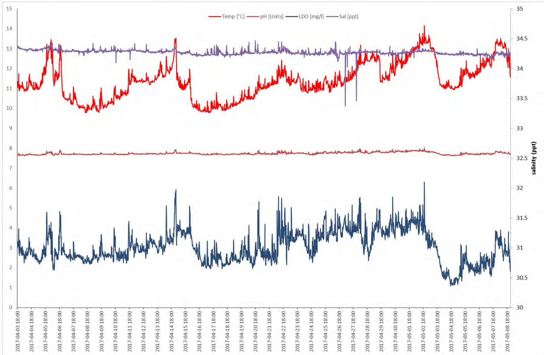
Figure 6.14. Temperature, salinity (sal), pH and dissolved oxygen (DO) recorded by the CTD deployed in 23 m water depth adjacent to the RO plant discharge at the base of the iron ore terminal.
