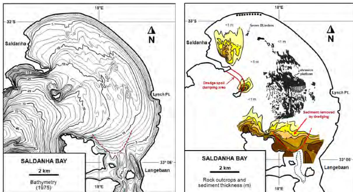
Figure 3.56. Ebb tide delta at the entrance to Langebaan Lagoon where sediment was dredged for construction of the causeway between Marcus Island and the mainland in the late 1970s. Source: Flemming (2016).
