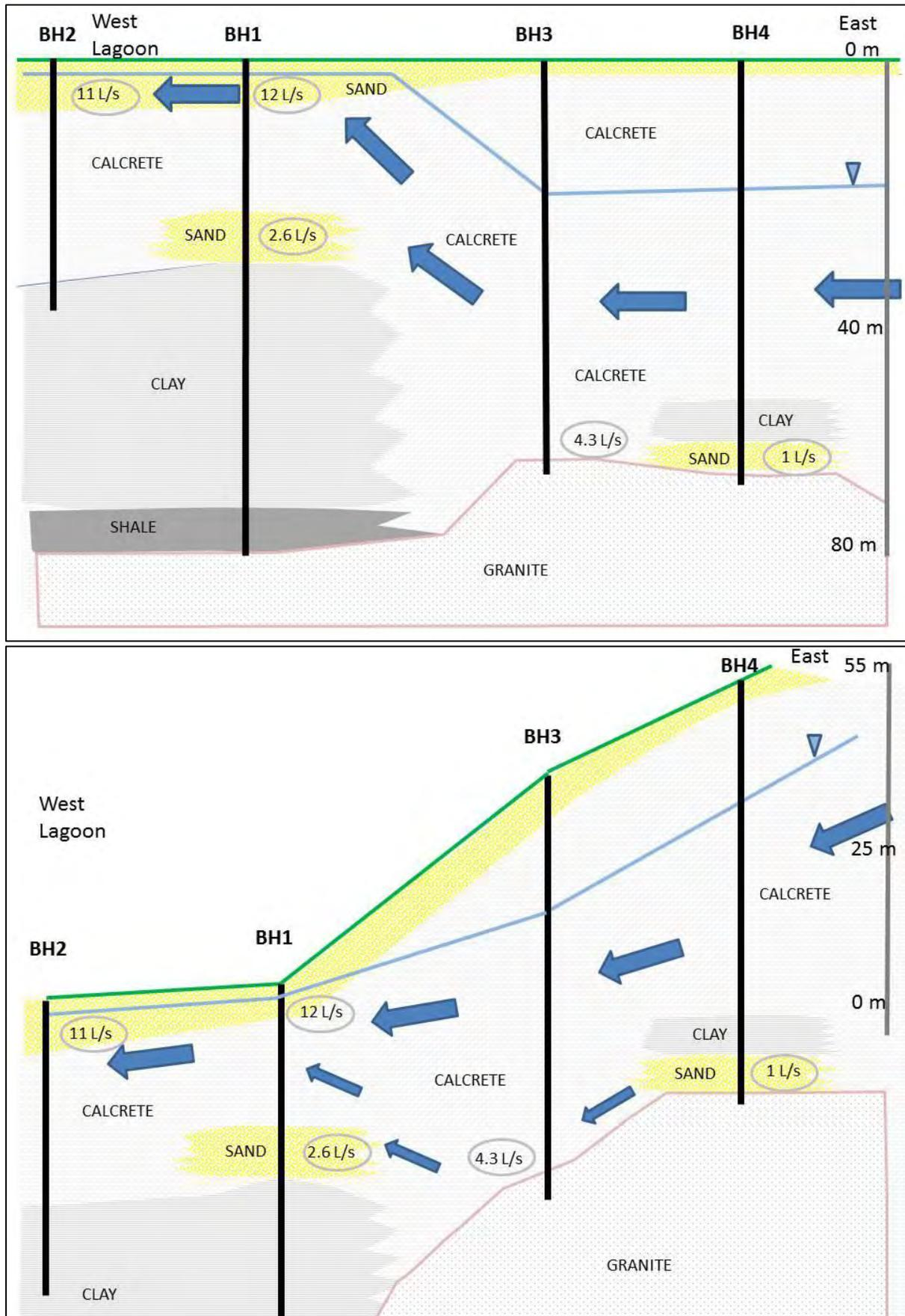
Figure 5.3 Geological cross-section of the Geelbek borehole (mbgl), showing ground at surface level (top) and corrected for elevation (bottom) (GEOSS 2014).
