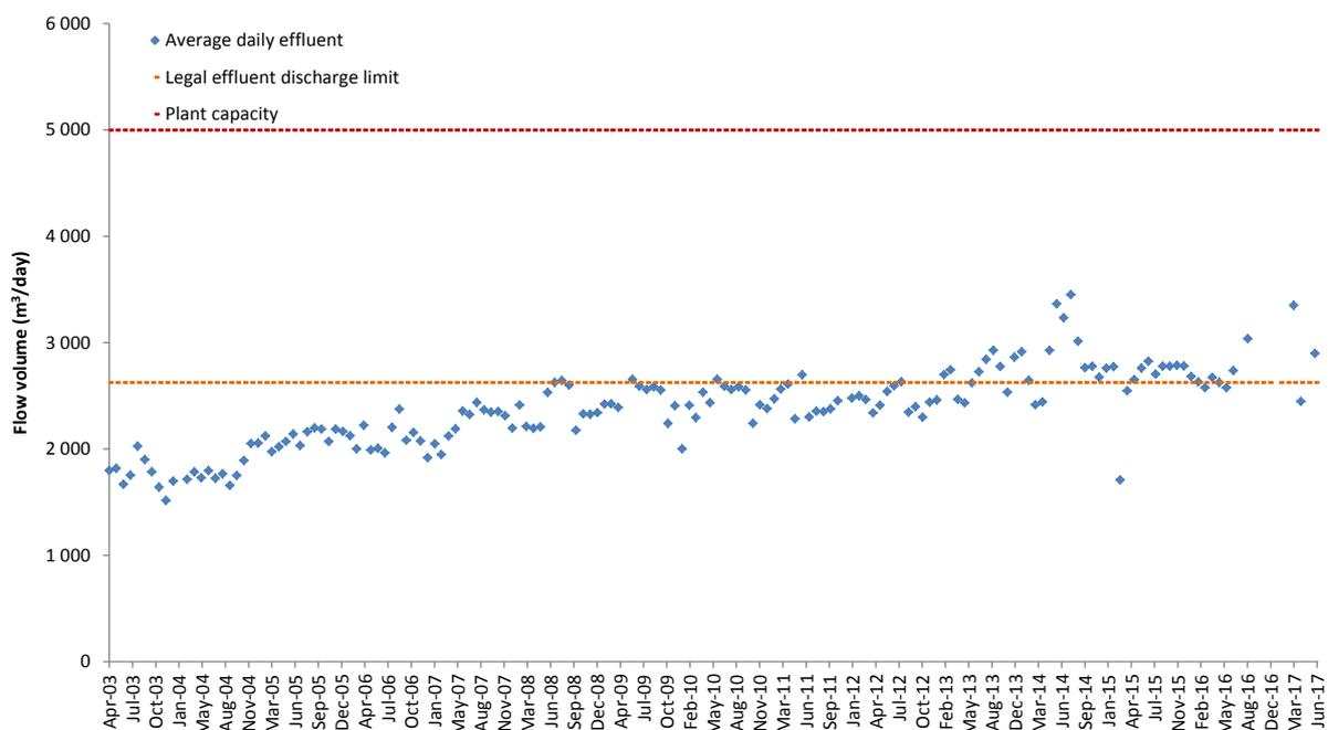
**Figure 3.23.** Trend in average daily effluent ( $\text{m}^3/\text{month}$ ) released from the Saldanha Wastewater Treatment Works, April 2003-June 2017. Allowable discharge limits in terms of the exemption issued by DWS under the National Water Act (No. 36 of 1998) are represented by the dashed orange line and the design capacity of the plant by the red line (Source: Saldanha Bay Municipality).
