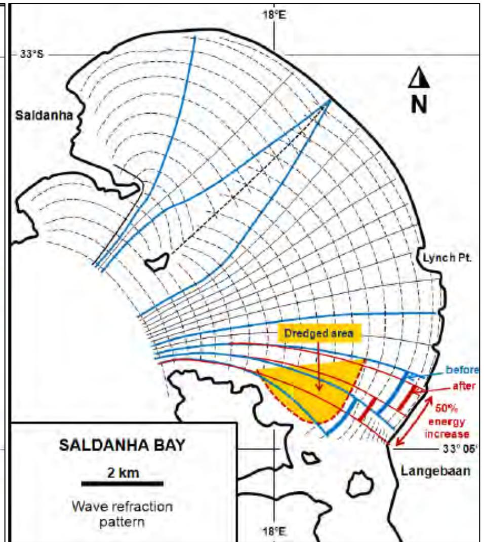
Figure 3.58. Changes in wave refraction patterns and a consequent increase in wave energy density at the shoreline at Langebaan Beach - a result of sediment removal during the construction of the causeway linking Marcus Island with the mainland. Source: Flemming (2016).
