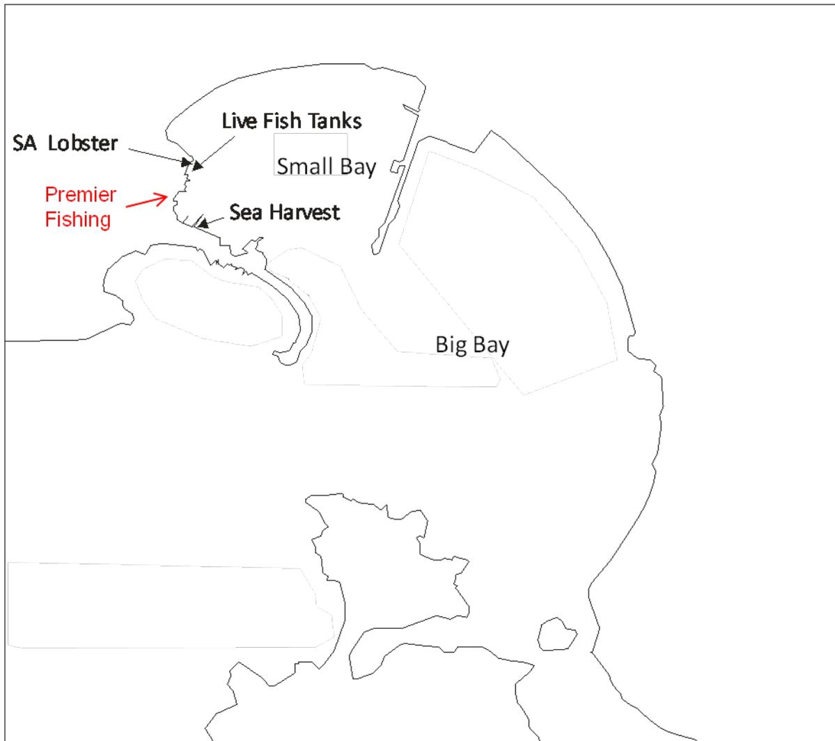
**Figure 3.43.** Location of seawater intakes and discharges for current and proposed seafood processing factories in Saldanha Bay. Current factories are indicated in black while the proposed Premier Fishing Fish Processing Plant is indicated in red.
