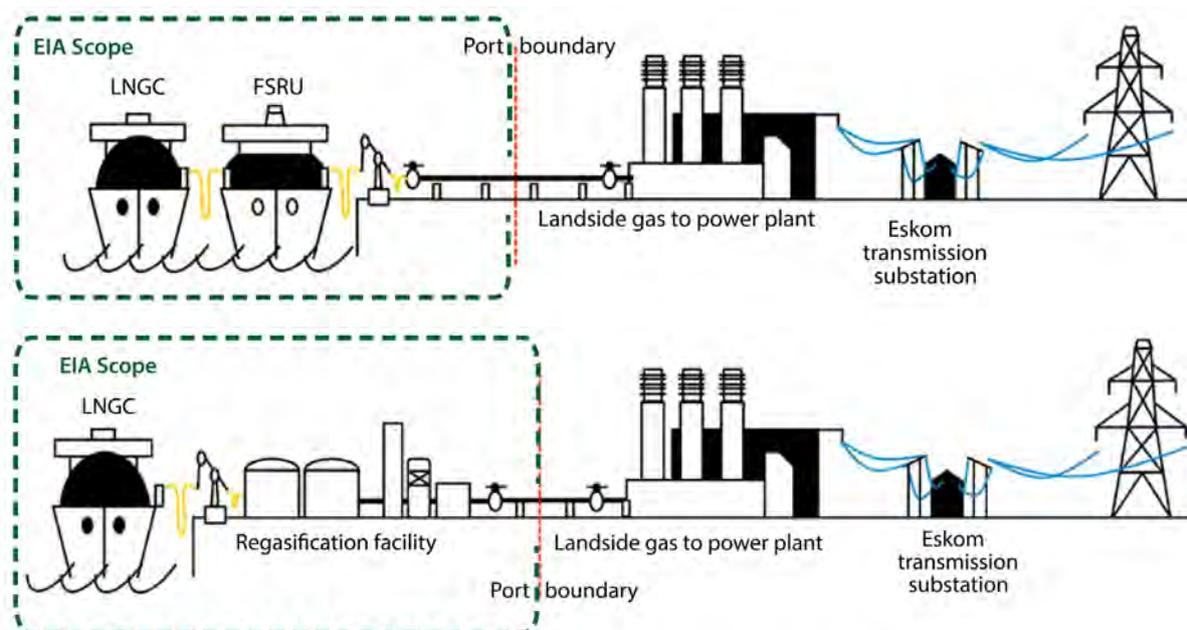
Figure 3.12 An illustration of the floating (top) and land-based (bottom) regasification technology (Source: Background Information Document, ERM 2015a).
