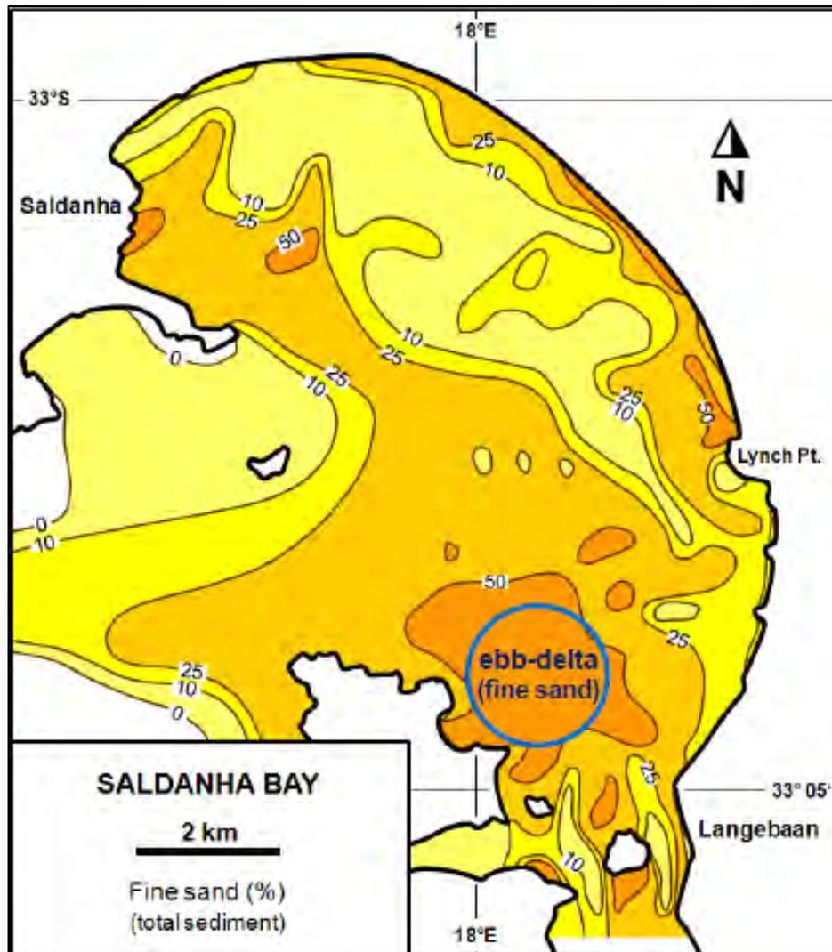
Figure 3.57. Ebb tide delta at the entrance to Langebaan Lagoon where sediment was dredged for construction of the causeway between Marcus Island and the mainland in the late 1970s. Source: Flemming (2016).
