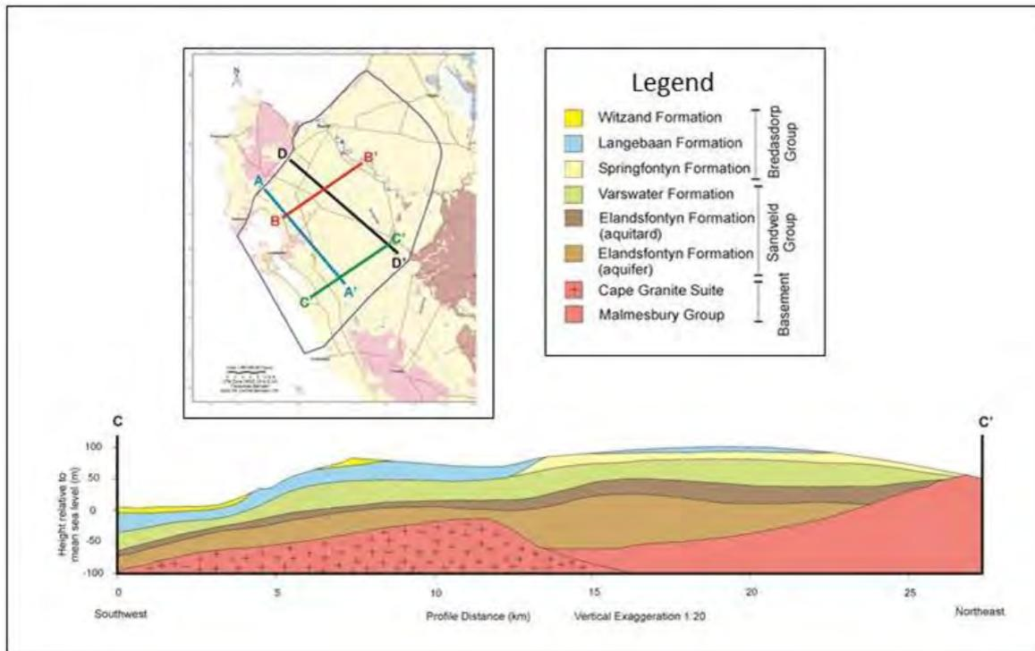
Figure 5.6 Geological cross-section (C-C') beneath the Geelbek area (DWAF 2008)
