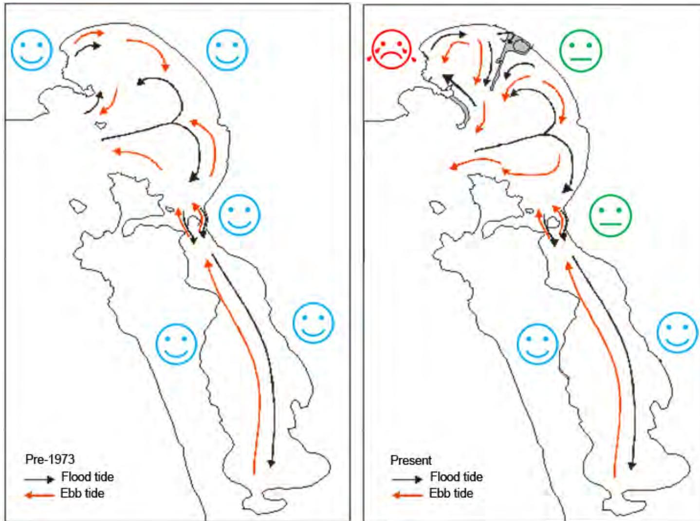
Figure 6.1 Schematic representation of the surface currents and circulation of Saldanha Bay prior to the harbour development (Pre-1973) and after construction of the causeway and iron ore terminal (Present) (Adapted from: Shannon & Stander 1977 and Weeks et al. 1991a).
