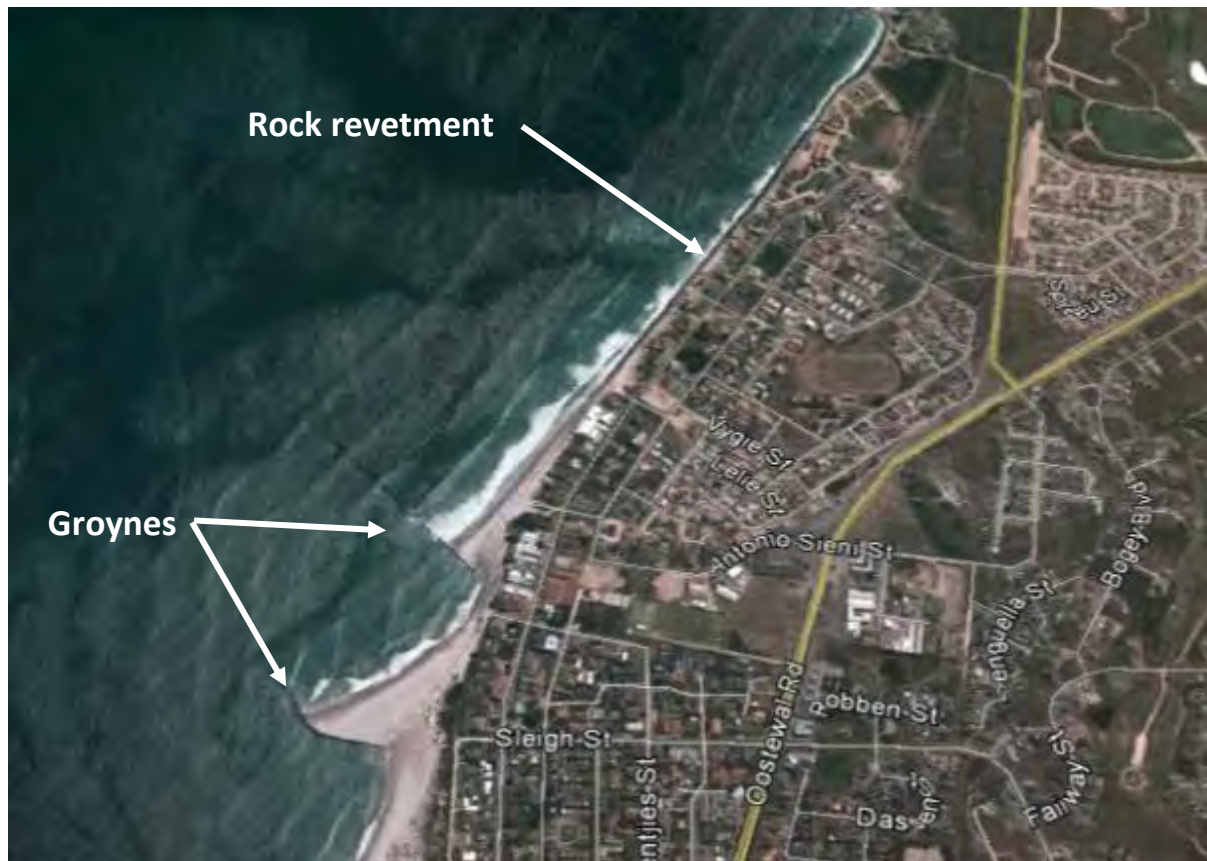
Figure 3.50. Groynes and rock revetment at Langebaan North beach. Source: Google Earth.
