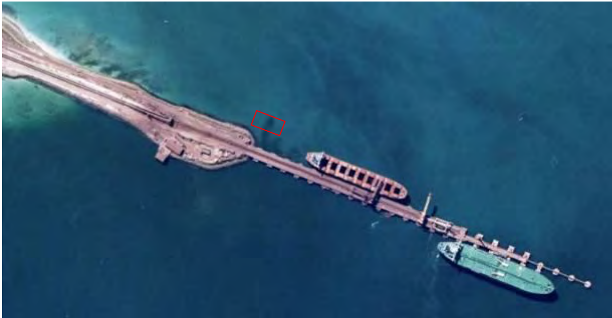
Figure 3.11. Location of the maintenance dredging site between Caissons 3 and 4 on the ore terminal.
