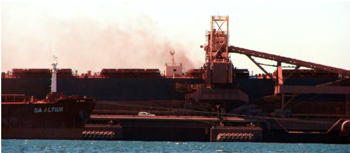
Figure 3.17 An iron ore vessel being loaded showing associated iron ore dust emission. Freshwater from the Transnet RO plant will be used to mitigate this impact by wetting the ore before loading.
