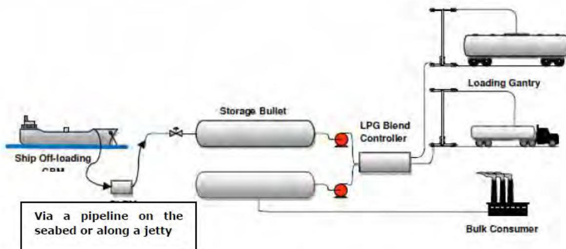
Figure 3.11. An illustration of an LPG transfer scheme (Source: ERM Final Scoping Report 2011)
