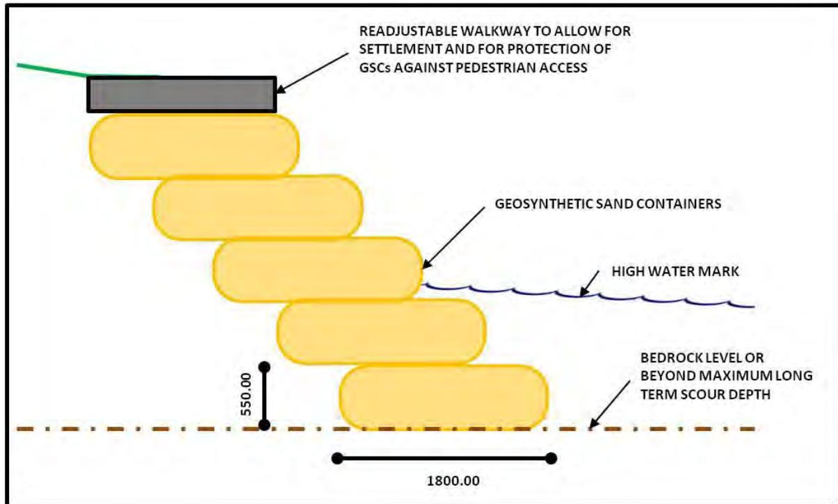
Figure 5.13. Design proposal 1 for the proposed Melck Street walkway: Geosynthetic Sand Container wall. Source: Common Ground Consulting (2013b).
