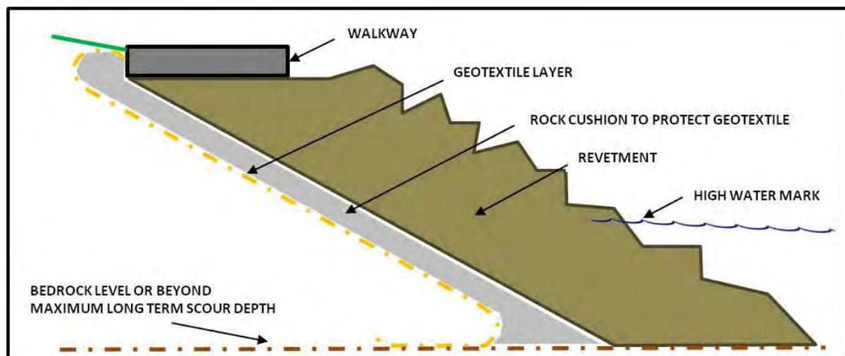
Figure 5.15. Design proposal 3 for the proposed Melck Street walkway: Rock revetment. Source: Common Ground Consulting (2013b).
