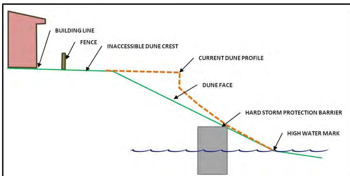
Figure 5.12 Submerged storm protection barrier proposed for Leentjiesklip Caravan Park (Common Ground Consulting 2013b).
