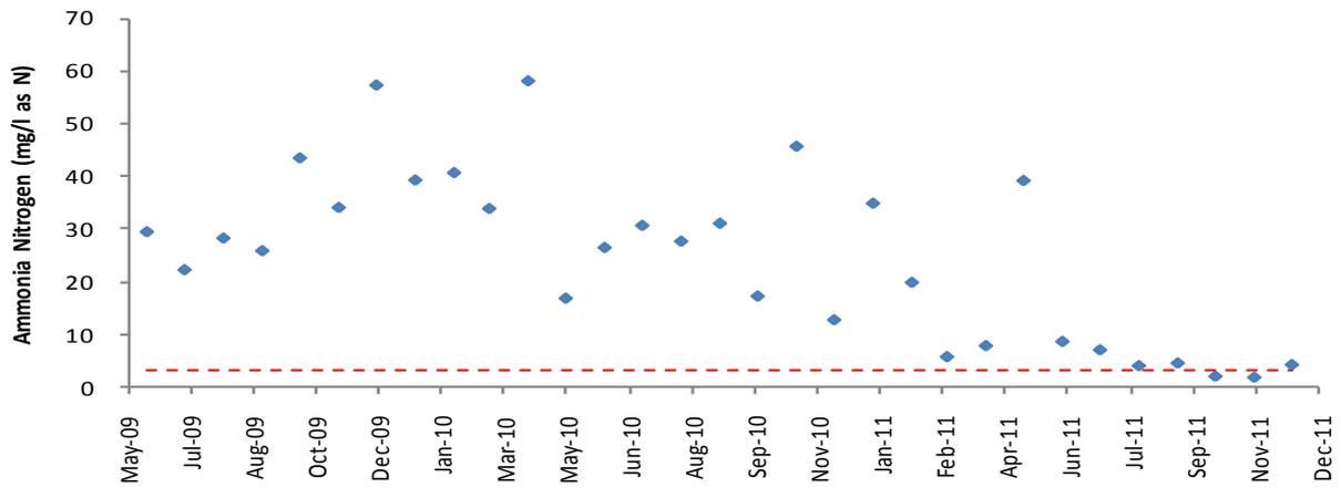
Figure 3.26. Monthly trends in the concentration of Ammonia Nitrate in effluent from Langebaan WWTW, June 2009 - December 2011. Allowable limits as specified in terms of a General Authorisation under the National Water Act 1998 are represented by the red line.
