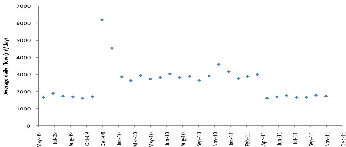
**Figure 3.22. Monthly trends in the daily volume of effluent discharged from the Langebaan WWTW in the period June 2009–November 2011.**
