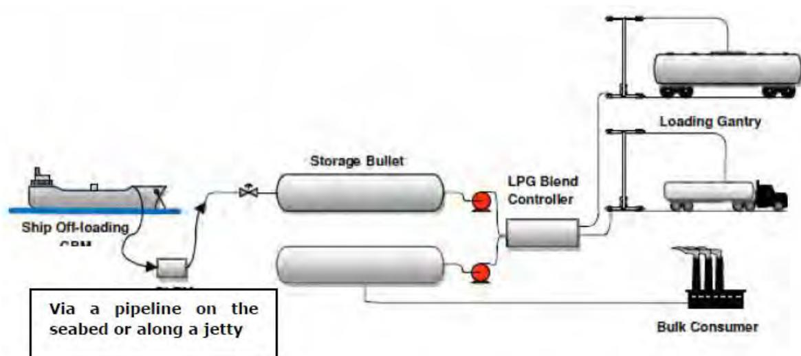
Figure 3.9. An illustration of an LPG transfer scheme (Source: ERM Final Scoping Report 2011)
