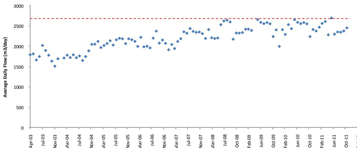
**Figure 3.14.** Monthly trends in the volume of effluent released from the Saldanha WWTW, Apr 2003-December 2011, and authorised total volume per year expressed as a daily limit (red line). Allowable discharge limits as specified in terms of the exemption issued by DWAF under the National Water Act 1998 are represented by the dashed red line.
