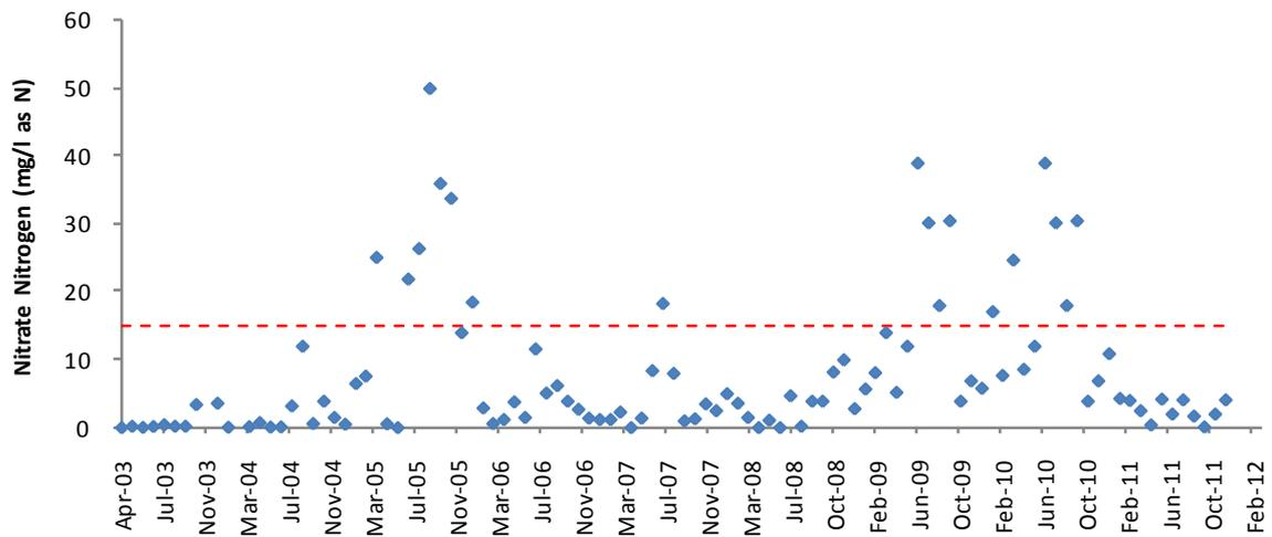
Figure 3.27. Monthly trends in the concentration of Nitrate Nitrogen in effluent from Langebaan WWTW, June 2009 - December 2011. Allowable limits as specified in terms of a General Authorisation under the National Water Act 1998 are represented by the red line.
