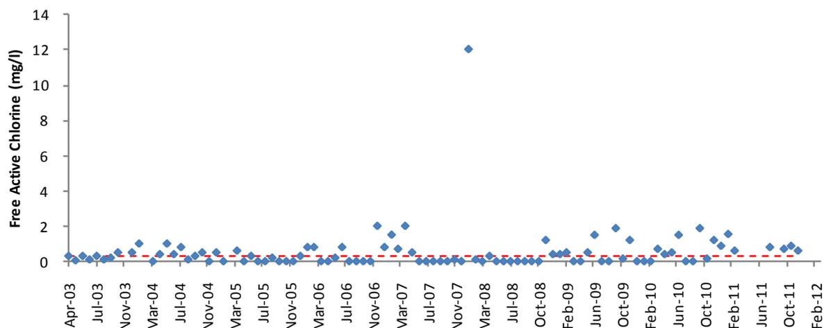
**Figure 3.29. Monthly trends in the concentration of Free Active Chlorine in effluent from Langebaan WWTW, June 2009 - December 2011. Allowable limits as specified in terms of a General Authorisation under the National Water Act 1998 are represented by the red line.**
