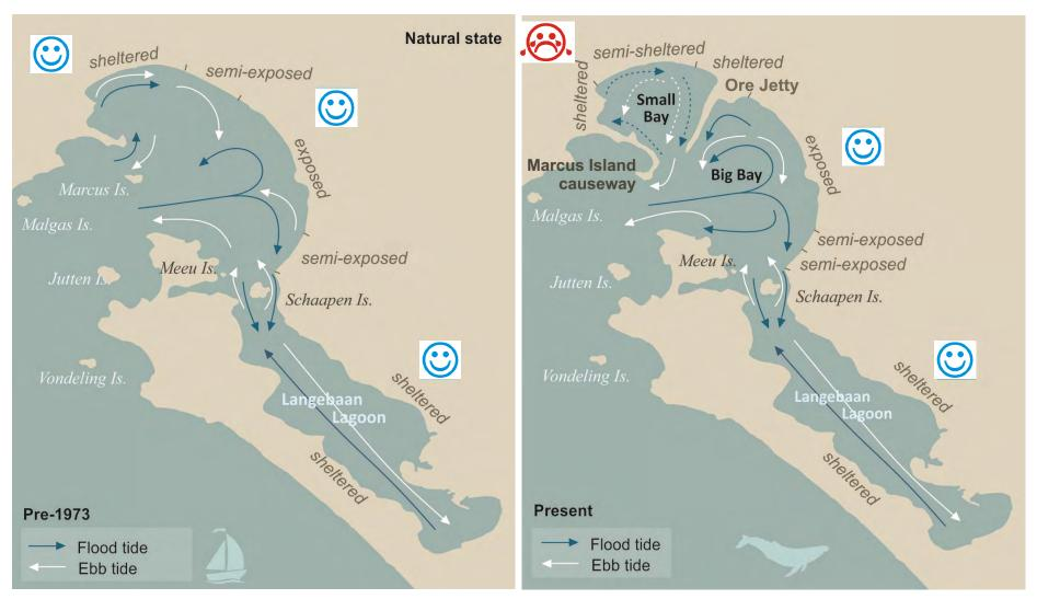
Figure 4.1. Schematic representation of the surface currents and circulation of Saldanha Bay (A) prior to the harbour development (Pre-1973) and (B) after construction of the causeway and iron-ore terminal (Present). (Adapted from Shannon and Stander 1977 and Weeks *et al.* 1991a)
