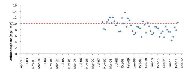
Figure 3.28. Monthly trends in the concentration of Orthophosphate in effluent from Langebaan WWTW, June 2009 - December 2011. Allowable limits as specified in terms of a General Authorisation under the National Water Act 1998 are represented by the red line.
