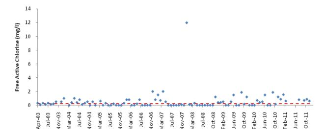
Figure 3.21. Monthly trends in Free Active Chlorine for effluent released from the Saldanha WWTW Apr 2003-December 2011. Allowable limits as specified in terms of a General Authorisation under the National Water Act 1998 are represented by the red line.
