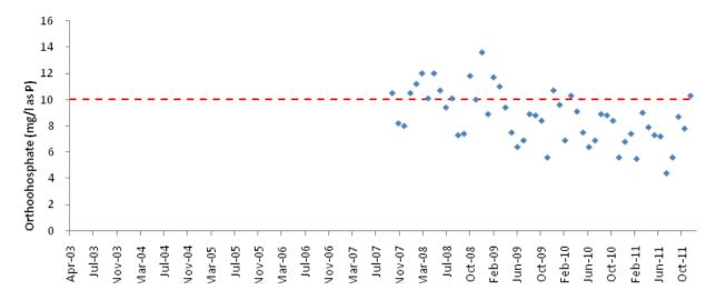
Figure 3.20. Monthly trends in water quality parameters Orthophosphate for effluent released from the Saldanha WWTW Apr 2003-December 2011. Allowable limits as specified in terms of a General Authorisation under the National Water Act 1998 are represented by the red line.
