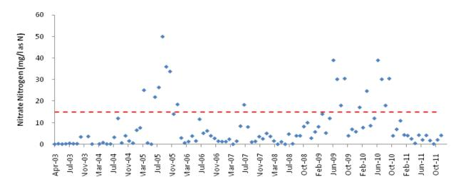
Figure 3.19. Monthly trends in Nitrate Nitrogen for effluent released from the Saldanha WWTW Apr 2003 -December 2011. Allowable limits as specified in terms of a General Authorisation under the National Water Act 1998 are represented by the red line.
