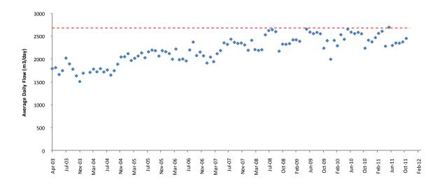
Figure 3.14. Monthly trends in the volume of effluent released from the Saldanha WWTW, Apr 2003-December 2011, and authorised total volume per year expressed as a daily limit (red line). Allowable discharge limits as specified in terms of the exemption issued by DWAF under the National Water Act 1998 are represented by the dashed red line.
