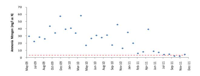
Figure 3.26. Monthly trends in the concentration of Ammonia Nitrate in effluent from Langebaan WWTW, June 2009 - December 2011. Allowable limits as specified in terms of a General Authorisation under the National Water Act 1998 are represented by the red line.
