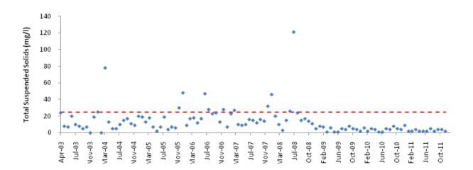
Figure 3.16. Monthly trends in the numbers of Total Suspended Solids in effluent released from the Saldanha WWTW, April 2003 - December 2011. Allowable limits as specified in terms of a General Authorisation under the National Water Act 1998 are represented by the dashed red line.
