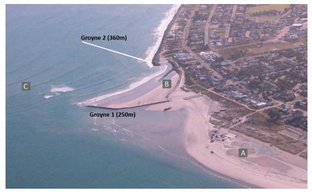
Figure 5.6 Groyne construction site Langebaan north beach. 1st groyne is completed and position of 2nd groyne is show in white. Area A and B are sand "slurry" sites (see text for explanation). Area C sand dredging site for beach reclamation. Source: Prestedge Retief Dresner Wijnberg.
