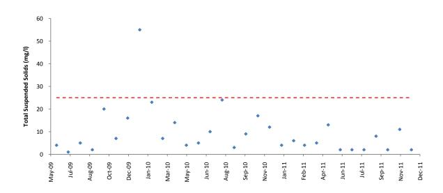
Figure 3.24. Monthly trends in Total Suspended Solids in effluent released from the Langebaan WWTW, June 2009 - December 2011. Allowable limits as specified in terms of a General Authorisation under the National Water Act 1998 are represented by the red line.
