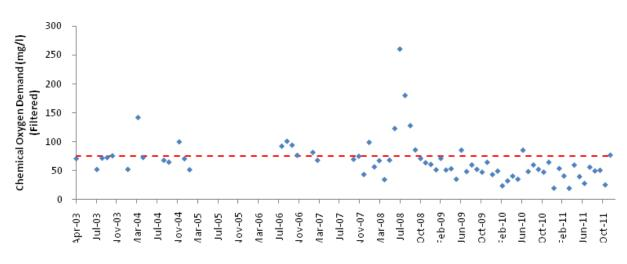
Figure 3.17.Monthly trends in the numbers of Chemical Oxygen Demand in effluent released from the<br/>Saldanha WWTW, April 2003 - December 2011. Allowable limits as specified in terms of a<br/>General Authorisation under the National Water Act 1998 are represented by the red line.
