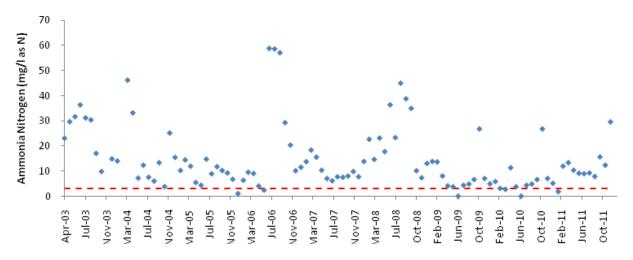
Figure 3.18. Monthly trends in Ammonia Nitrogen for effluent released from the Saldanha WWTW Apr 2003-December 2011. Allowable limits as specified in terms of a General Authorisation under the National Water Act 1998 are represented by the red line.
