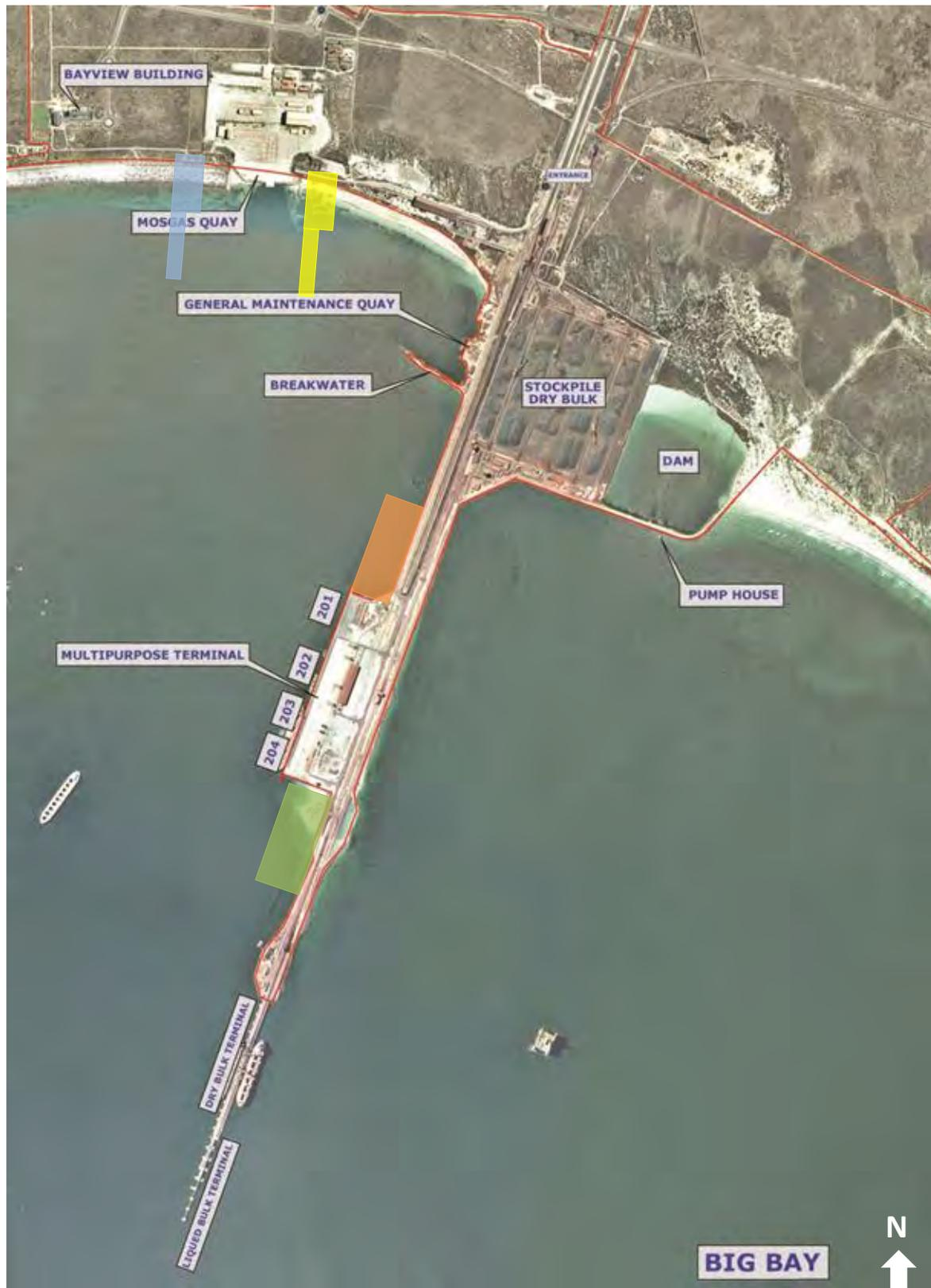
Figure 3.11 The iron ore terminal (IOT), the multi-purpose terminal (MPT), the Dry Bulk Terminal (DBT) and the Liquid Bulk Terminal (LBT) separating Big Bay and Small Bay. The preferred (green) and alternative (orange) position of the Berth 205 VRF and the preferred (yellow) and alternative (blue) options for the proposed Mossgas Jetty are indicated (Adapted from: ARUP 2016).
